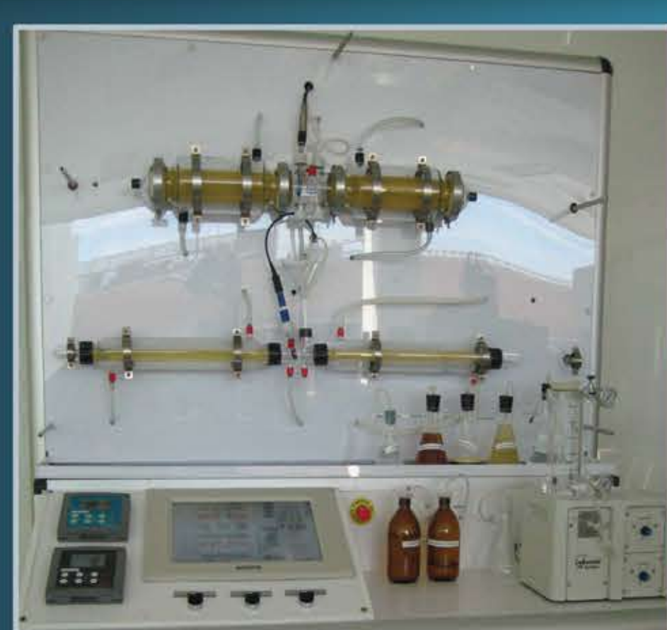
Image of In vitro Dynamic Gastrointestinal Digester (DGD) developed at AINIA Technologic Centre.
